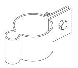
Strap type cable or point holder for use on vertical or horizontal pipe run – copper holder made of tinned copper strap 1" wide, 0.064" thick – aluminum holder made of aluminum strap 1" wide, 0.080" thick – furnished with 1" long bronze or stainless steel bolt and nut for tension on pipe – for main sized cables through No. 605 and point diameters 3/8" to 5/8" – various pipe sizes available on request.
