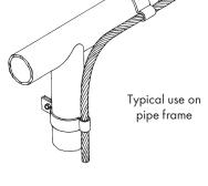
Strap type cable or point holder for use on vertical or horizontal pipe run – copper holder made of tinned copper strap 1" wide, 0.064" thick – aluminum holder made of aluminum strap 1" wide, 0.080" thick – stand-off distance 1" from wall of pipe – furnished with 1" long bronze or stainless steel bolt and nut for tension on pipe – for main sized cables through No. 605 and point diameters 3/8" to 5/8" – various pipe sizes available on request.
